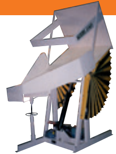
STATIONARY DUMPER WITH ADJUSTABLE CHUTE ATTACHMENT AND SAFETY SKIRTING
