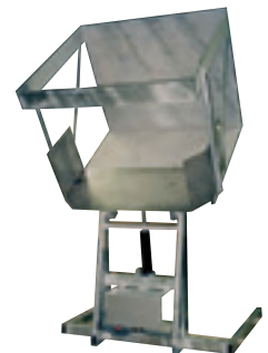
GALVANIZED DUMPER WITH STAINLESS CHUTE
